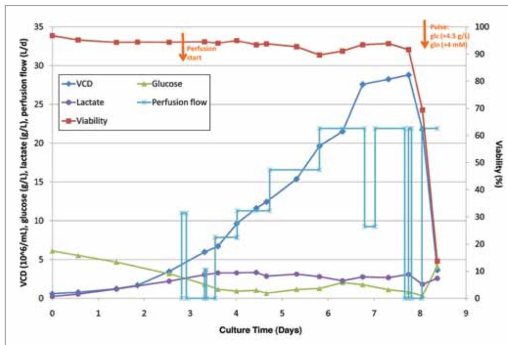
**Figure 1.** Perfusion matched with PBS Biotech bioreactors. Perfusion is seen to help sustain cell viability and boost cell density, while keeping lactate waste levels low.
